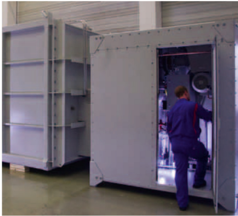
DFC@250 EU MCFC-Fuel Cell Power Plant 250 kW; 400 V; 50 Hz
